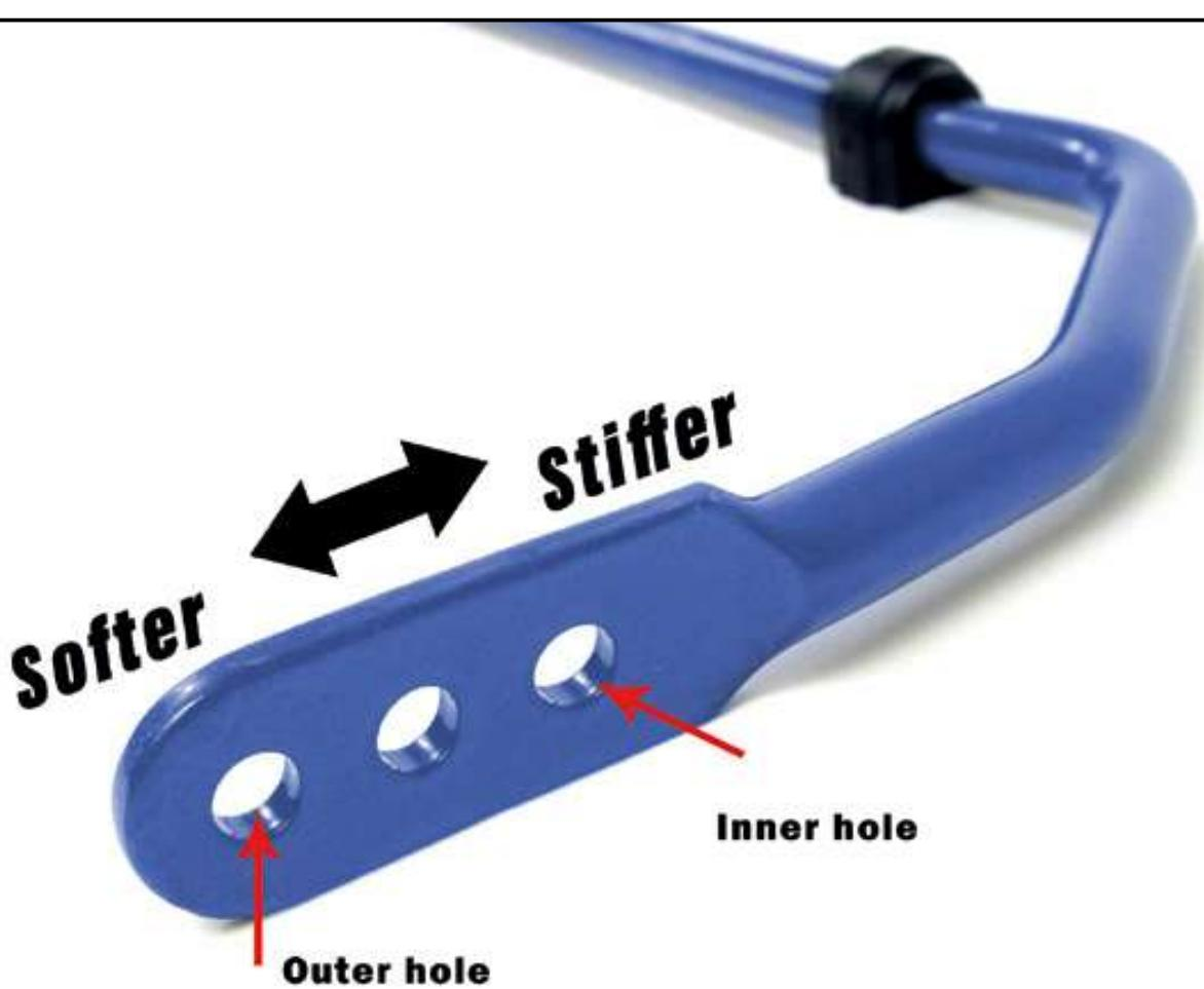
H&R anti-roll bars have a higher stiffness than the OE anti-roll bars. Wherever possible, multiple adjustment holes are provided.
