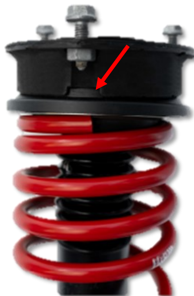
Abb. 6: Position Federende Fig. 6: position spring end
