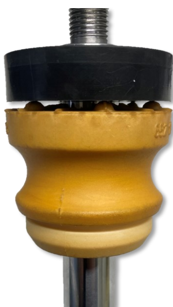
Abb. 2: VA Anschlagpuffer Fig. 2: FA bump rubber
