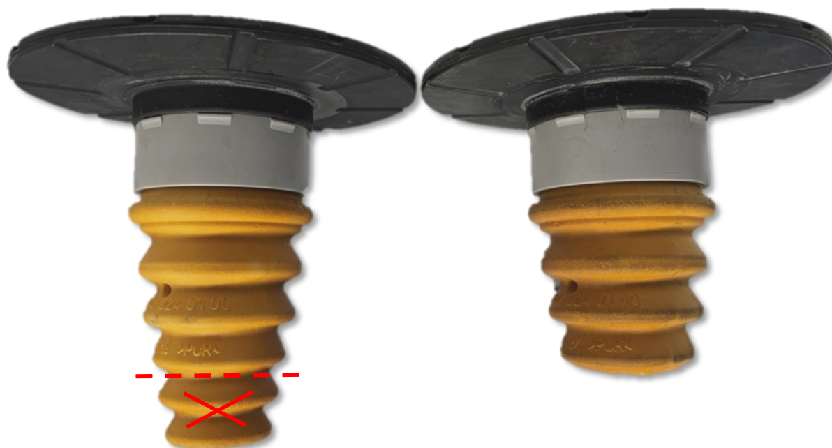
Abb. 5: Puffer kürzen Fig. 5: shorten bump rubber
