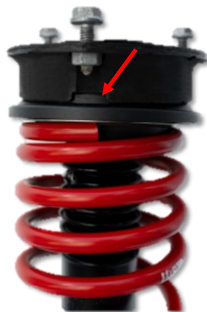
Abb. 4: Position Federende Fig. 4: position spring end
