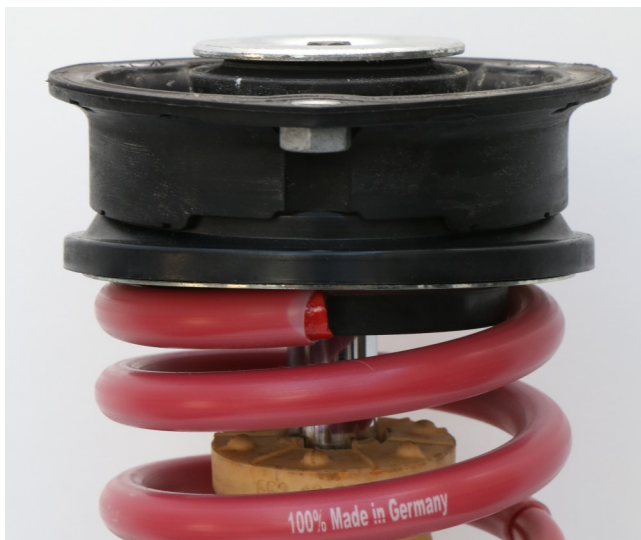
Abb. 1: Position Federende beachten Fig. 1: Ensure position of the spring end
