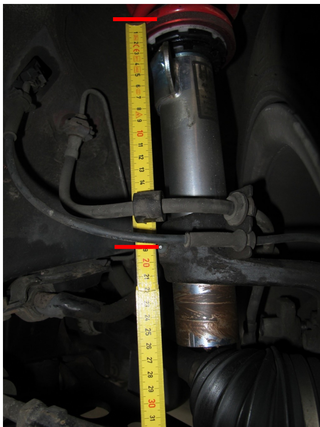
Fig. 1: FA spring plate adjustment dimension
