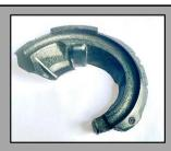
Eibach recommends replacing the lower spring seat (OE-No. 500 412 545 D) where the front spring locates on the damper whenever new front coil springs are installed.
