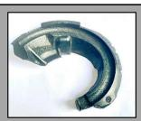
Eibach recommends replacing the lower spring seat (OE-No. 5QO 412 545 D) where the front spring locates on the damper whenever new front coil springs are installed.
